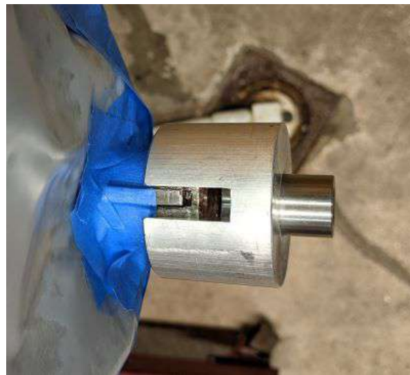
Another view of snout tool on crankshaft
