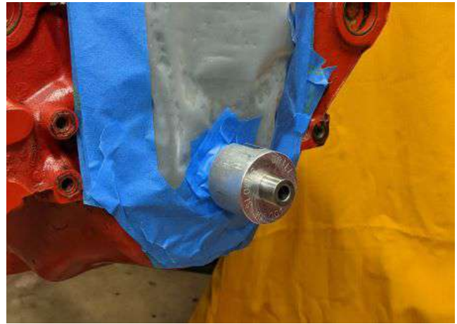
Snout tool secured on crankshaft
