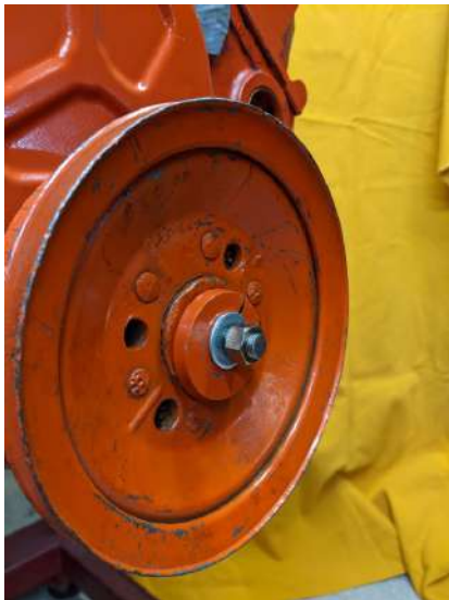
Using a threaded rod to install balancer on crank
