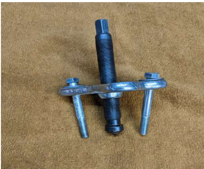
Typical puller that threads into the balancer
