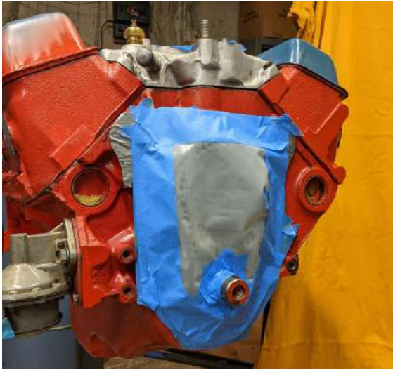
Plastic and tape to cover front of engine
